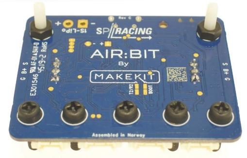
Mount the micro:bit on top with 5 nuts.
